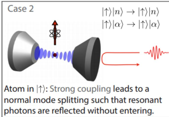
Due to destructive interference on the coupling mirror:  $\pi$  phase shift [5, 6] on the total wavefunction whenever a single photon can enter the cavity, i.e. the atom is not coupling ( $|\downarrow\rangle$ ).
