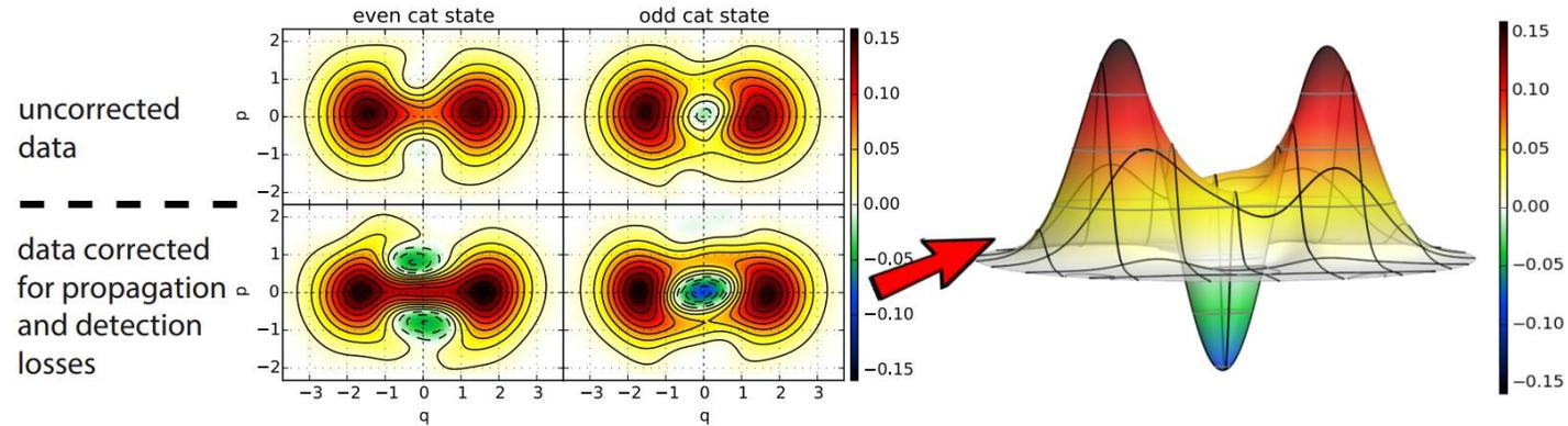
Losses limit the size of the cat states with negativity: Cavity losses: 19%. Propagation and detection losses: 25%
