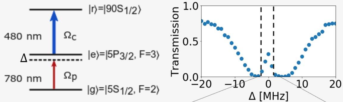
**B)** The cloud is transparent to probe photons.
