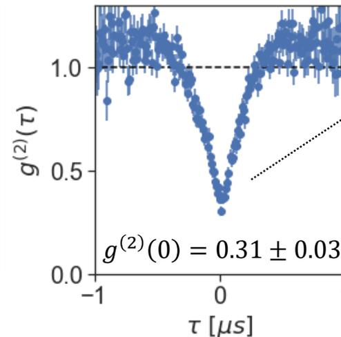
**C)** “Common” **Rydberg EIT antibunching** [4]: Only one photon leaves the medium at a time, delocalized within the output pulse
