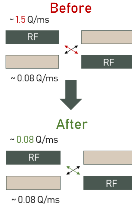
Side view of the Paul trap with heating components along the RF and DC electrodes
