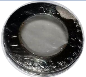
Fig.1 CNT film on the aperture (aperture diameter 5 - 8 mm)
