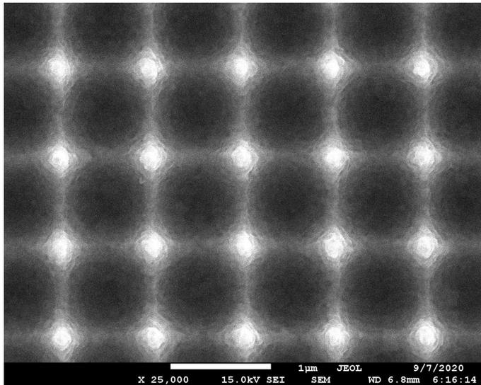
Fig. 3 SEM image of the substrate coated with silver film
