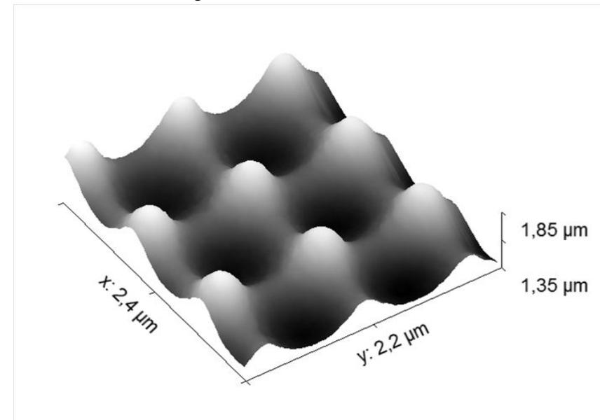
Fig.1 AFM data from the dielectric glass substrate before silver coating and nanostructuring
