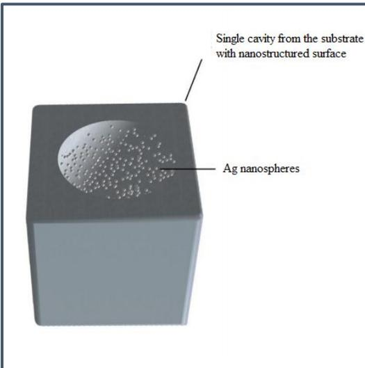
Fig. 3 Model of obtained nanostructures on the substrate
