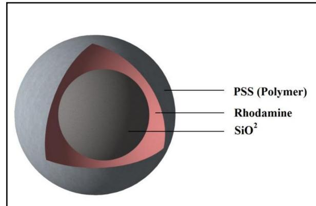
Fig.4 Model of the microcapsule with a Raman active label
