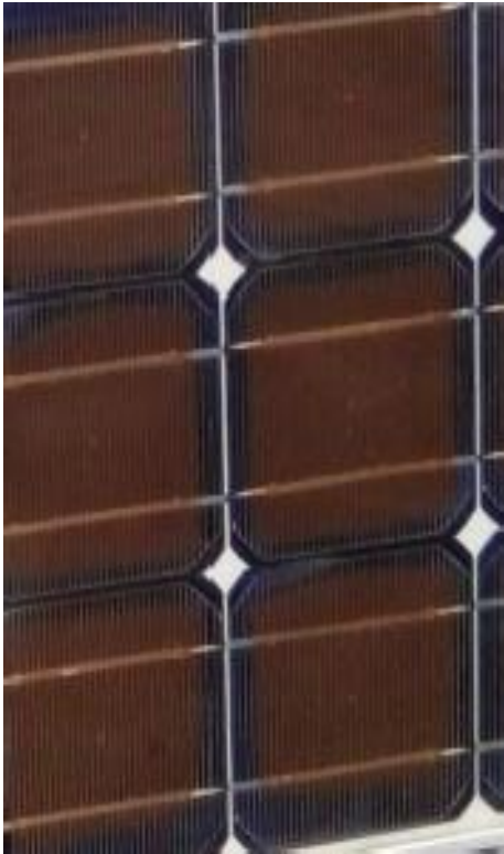
Fig .2 Discoloration of the EVA “Browning”.
